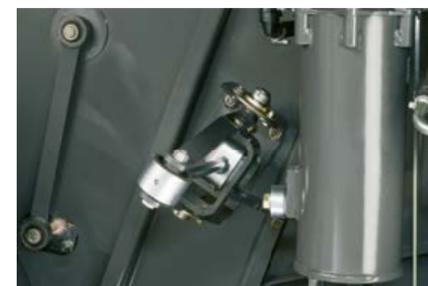
With its combination of hydraulic and mechanical elements, the fully automatic 3D cleaning system is able to dispense completely with electronic sensors.
