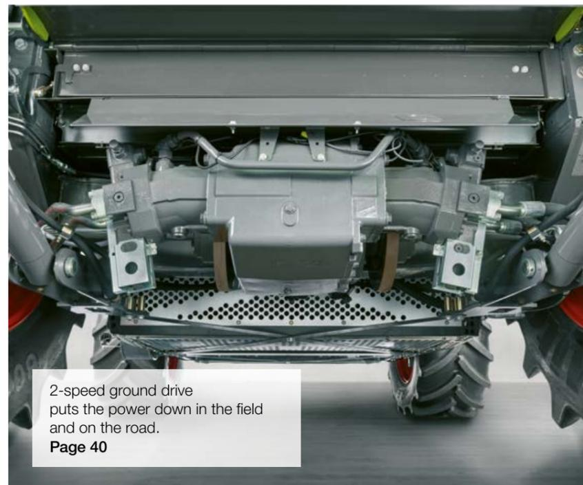
2-speed ground drive puts the power down in the field and on the road.
