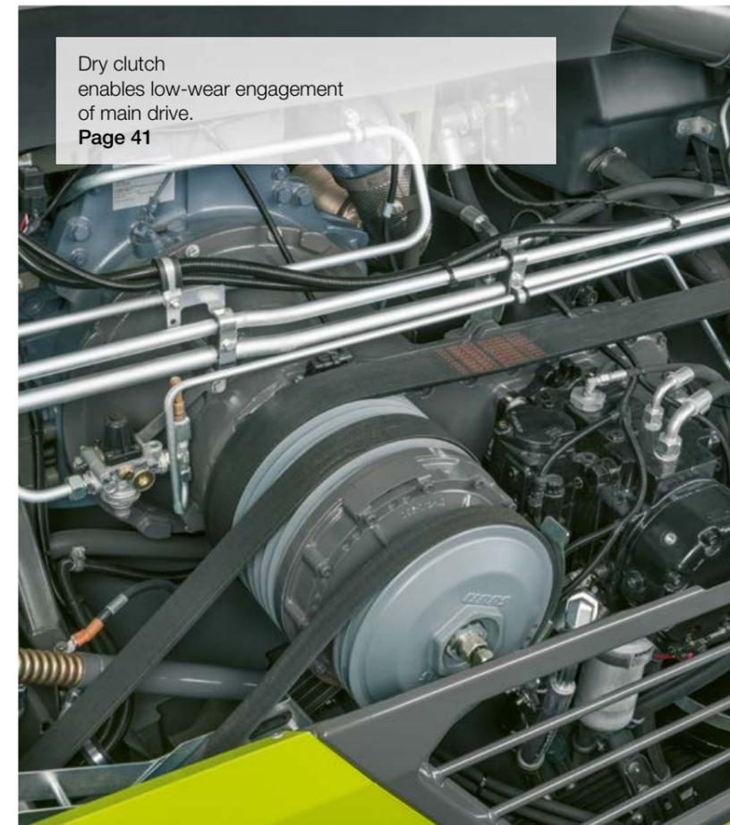
Dry clutch enables low-wear engagement of main drive.
