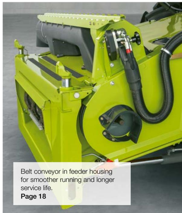
Belt conveyor in feeder housing for smoother running and longer service life.
