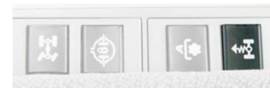
Switch to activate front axle suspension.
