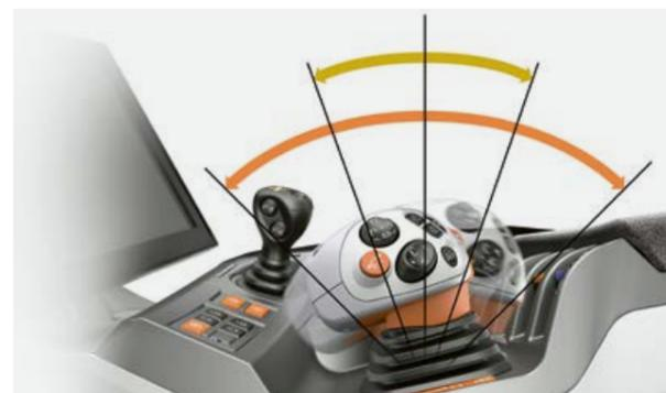
Shifting operation Powershift speeds + / -      Shifting operation Range + / -
