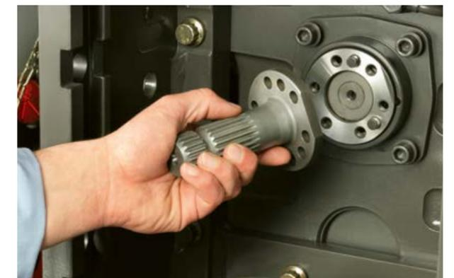
The PTO stub can be changed easily.
