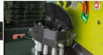
With the FITLOCK and MACH coupling systems, you only need to dismount once when attaching or removing the front loader.
