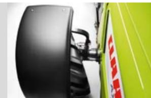
Pivoting front mudguards allow maximum steering angles.
