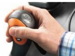
The TWINSHIFT function is pushbutton-operated via the shift lever. The activated level is displayed on the instrument panel.
