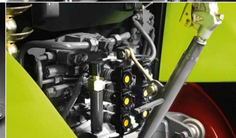
The PTO stub can be changed quickly (dry state) by removing six bolts, enabling the AXOS to power a huge variety of attachments.
