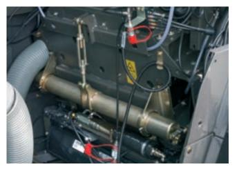
This results in a huge reduction in the amount of energy required. If, for example, very dry grass requires a high discharge rate, a very narrow clearance setting is required. This can even be set up in CEBIS while travelling and then applied automatically at the start of the chopping process.
