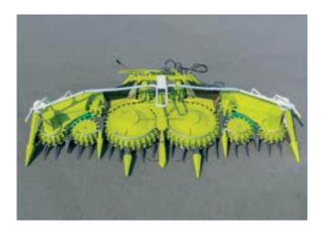
NEW: The ORBIS 600 SD is offered in parallel to the ORBIS 600. The SD is particularly suited to normal and low-growing stands. The outer sections with the small discs and the additional vertical feed drums enable an extremely good crop flow. It is also possible to cut the stubble extremely close.
