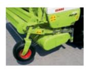
Hydraulically folding castor guide wheels
