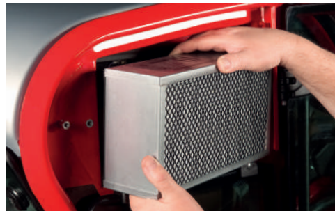
Large filters with quick and immediate access for ordinary maintenance.
