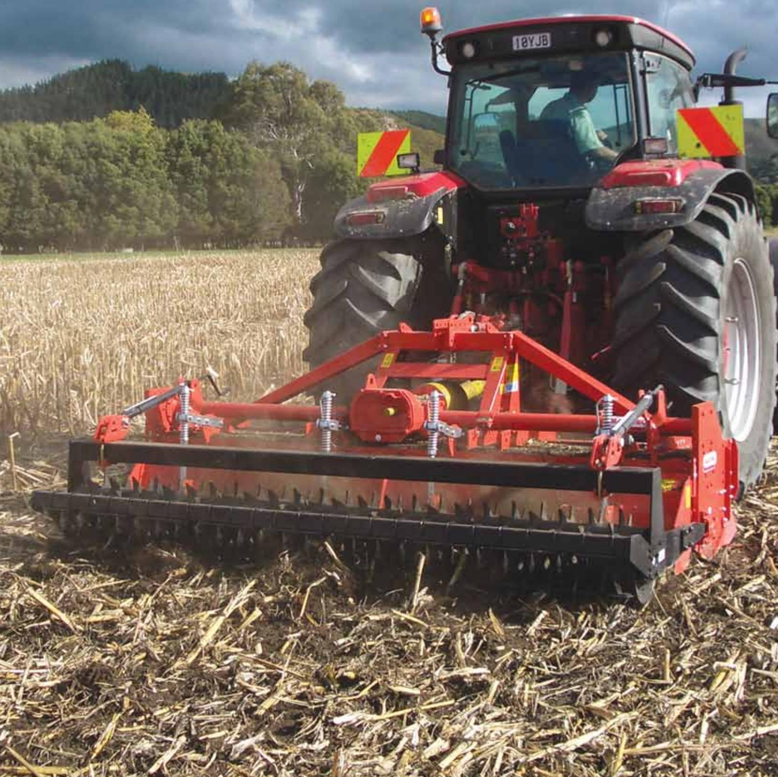
The Maschio Condor is a rugged and versatile cultivation machine that is used predominantly as a single pass unit. The spiked rotor design allows the condor to handle trash and stones with ease providing a well cultivated seed bed in one pass in most soil conditions. Unlike a rotary hoe the spiked rotor concept eliminates problems associated with panning.
