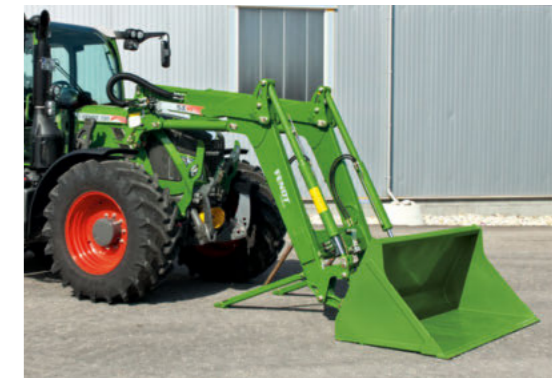
Fendt Cargo-Lock guarantees quick and easy mounting and removal. A multi-coupler connects all hydraulic and electric lines at once – even under pressure on the front loader side.
