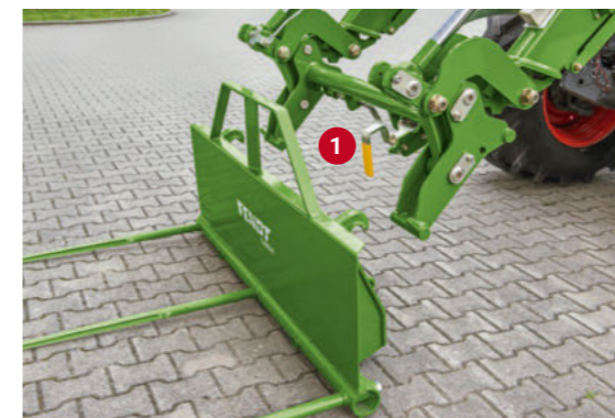
The implement is conveniently unlocked using a lever (1) on the quick-attach frame; it just takes a flick of the hand. When mounting an attachment, lock it automatically by tipping it back completely.
