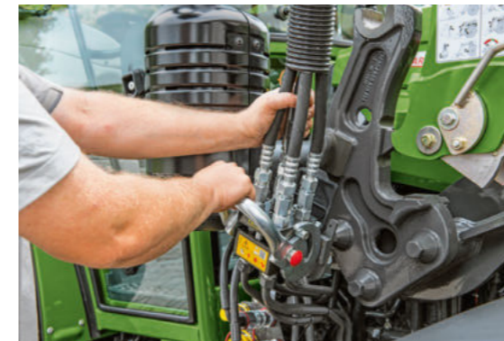
The new Fendt Cargo-Lock makes mounting and removing the loader easy and fast. The multi-coupler also saves time. It means you can connect all electric and hydraulic lines with just one hand movement.
