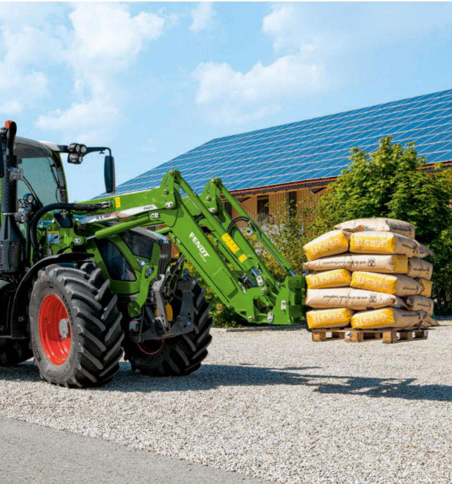
All hydraulic components are fitted in the cross beam and are therefore fully protected from dirt and mechanical damage.
