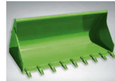
The heavy material bucket is available in widths of 1600 mm (0.53 m³ flush volume) and 2000 mm (0.67 m³ flush volume). The bucket trough is rounded and smooth to prevent crop from sticking. The blades are made from hardened, low-wear high carbon steel and are 150 x 20 mm. They also include industrial loader tines which are bolted flush onto the underside of the blades, therefore preventing grooves during levelling.
